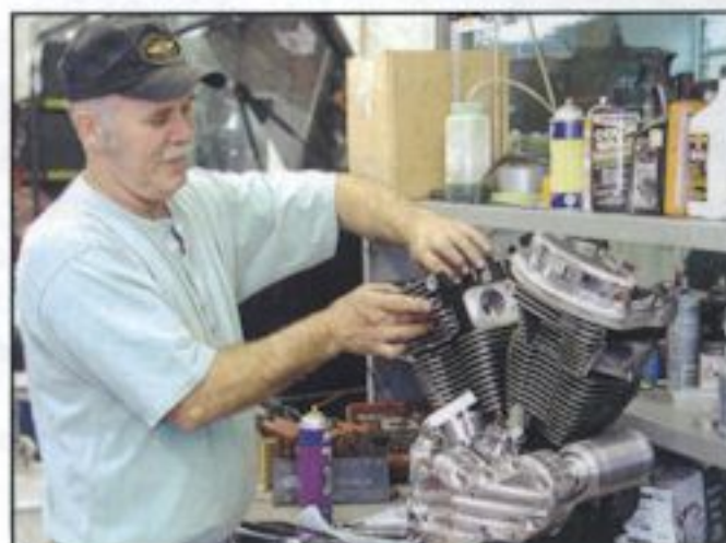
Here, Jesse's buttoning up one of our 96-in. engines with an Xzotic Panhead conversion.
