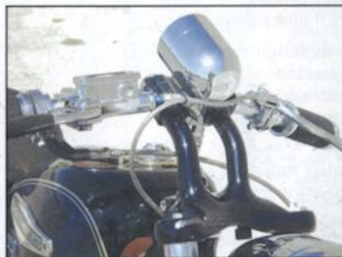
The one-piece riser-triple-tree is very nice indeed. The gas tank with the built-in ignition switch is a '50's H-D Hummer piece that Jesse found on E-Bay.
