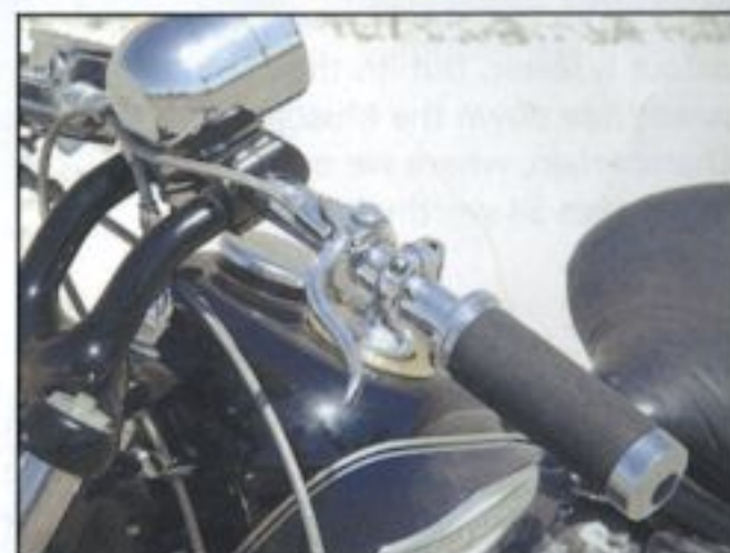
The sexy little Speed-E-Shift clutch lever is used only for starting and stopping.
